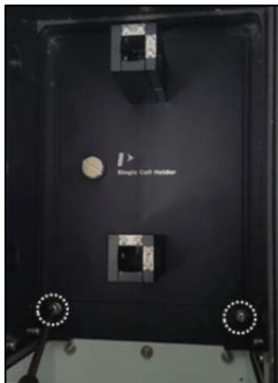
Figure 5 Location of the Phillips round head screws with washer
