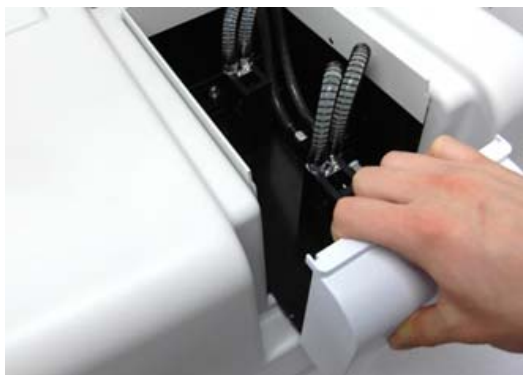
Figure 7 Inserting the Water Jacketed Single Cell Holder
