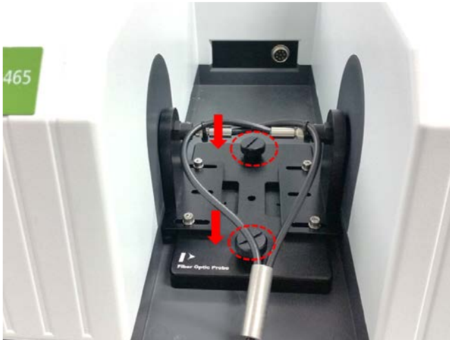
Figure 4 Installing the fiber Optic probe
