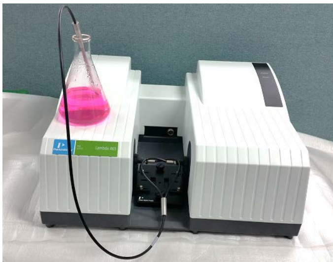
Figure 5 Placing the probe in the liquid
