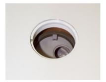
This exposes the reference pan position. The sample pan position is the one closer to the side of the instrument. The reference pan position is closer to the center of the instrument.
