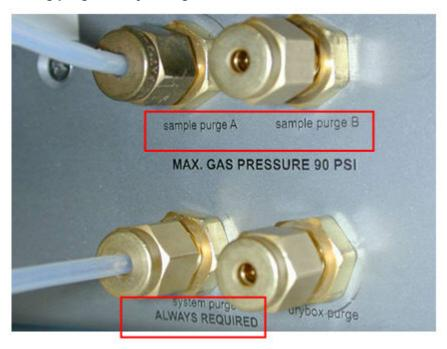
**NOTE:** The dry box purge inlet is only used when an autosampler is installed on the instrument.
