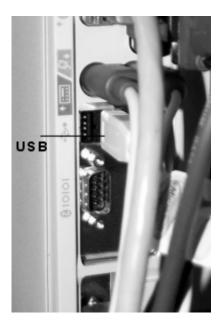
2. Attach the other end of the connector cable to the USB port on the EdgePort.
