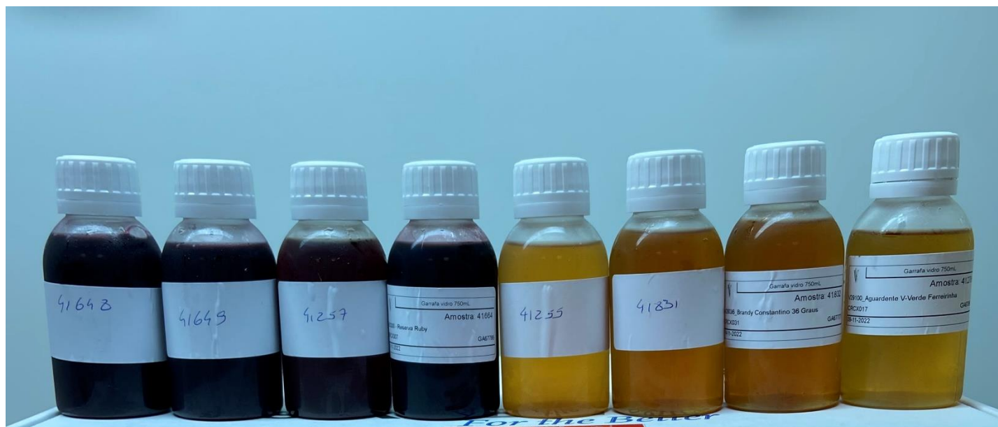
8 alcoholic beverages for sample analysis of higher alcohols by TVT-GC-FID
