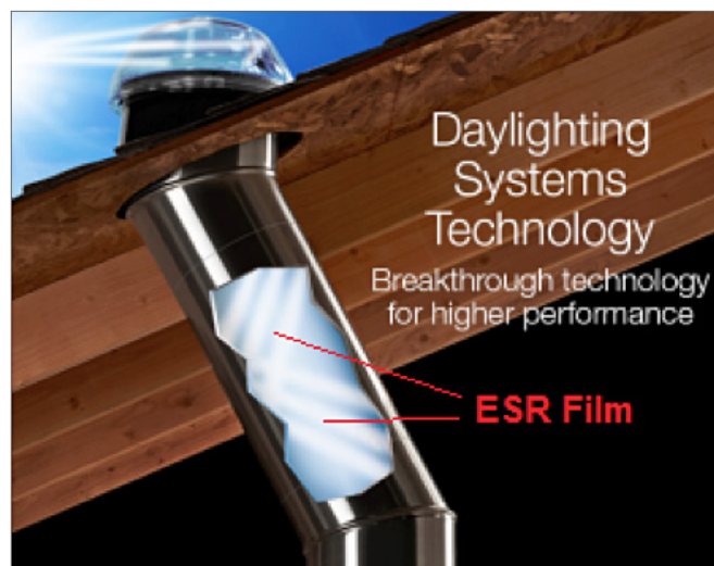
Figure 3. Example of Tubular Daylighting Devices (TDDs) which capture sunlight using a rooftop dome, and then transfer it indoors through a reflective tube that runs from the roof to the ceiling. For most commercial TDDs, ESR film is used in the interior of the light transfer tube to achieve high specular reflectivity (up to 99.7% reflective in the visible spectrum) thereby delivering maximum visible light.
