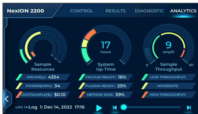
Figure 6. Example of LCD touchscreen, displaying Analytics window.
